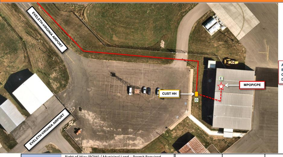
A TO B BORE & PL. 1.25" CONDUIT W/72CT 800FT в то с BORE & PL. 1.25" CONDUIT W/72CT 145FT C TO D BORE & PL. 1.25" CONDUIT W/24CT 840FT D TO E **PLACE 24CT IN EX. CBO** 175FT
