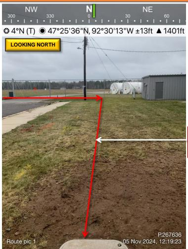
**LUMEN TO: BORE & PLACE 850FT OF NEW** 1.25IN CONDUIT & PULL NEW 24CT FIBER FROM HH-4280 MILLER TRUNK RD-2 (09+45) TO CUST HH (17+95).
